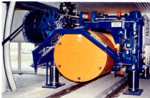
Waste Emplacement Machine
