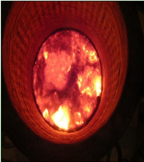
Molten glass inside the CIAE cold crucible melter in operation
